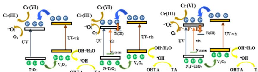
**Fig. 8.** Proposed mechanism for the photocatalytic reduction of Cr(VI) and photocatalytic oxidation of organic compounds by  $\cdot\text{OH}$  radical generation for the studied  $\text{V}_2\text{O}_5/\text{TiO}_2$ ,  $\text{V}_2\text{O}_5/\text{N-TiO}_2$  and  $\text{V}_2\text{O}_5/\text{N,F-TiO}_2$  photocatalysts.
