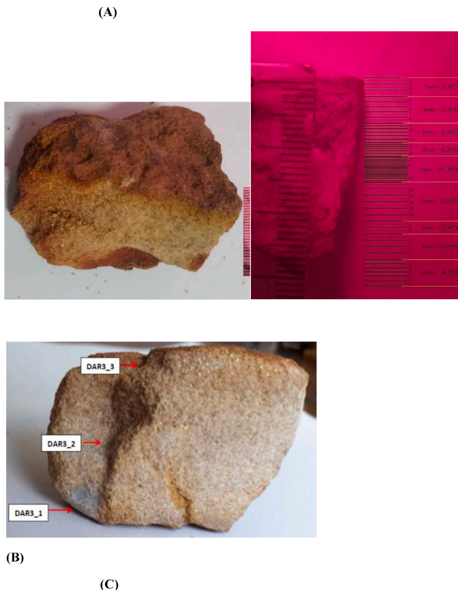
Fig. 3. Sampling for OSL: (a) the DC-3 sandstone sample with reddish weathered surfaces and the main stone body in yellow, and besides the profile of layers removed, (b) Macroscopic appearance of the sample DC-3. The labels DAR3-1, 2,3, indicate the three qualitatively different subdomains where further micro-sampling has been performed for mineralogical and chemical composition under X-ray techniques (X-ray powder diffraction and X-ray fluorescence analysis).
